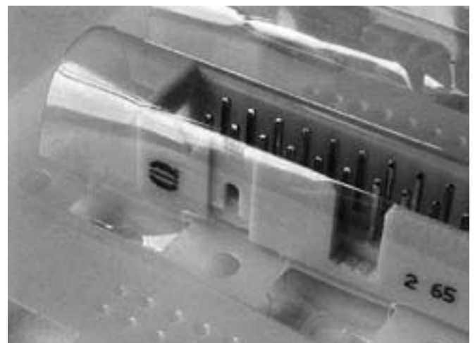
SEK connector mounted in a tape ready for placement using an odd form assembly station.
