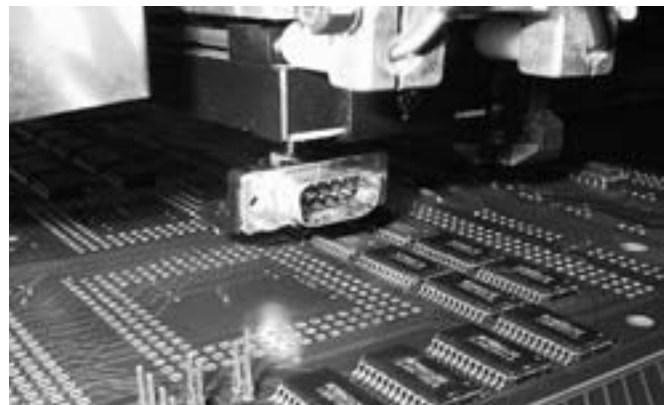
D-Sub in pick and place machine equipped with vacuum nozzle
